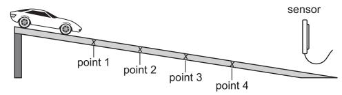
Aiden used a sensor to measure the speed of the car at the same location after the car was released from each point. Aiden concluded that the car had the most energy when it was released from point 1.
